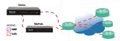
If it is not possible to use CISCO IP SLA for point-to-point network readings, Telcomanager offers its own probe as a solution, called TelcoProbe (all Telcomanager appliances can be configured as TelcoProbe). With TelcoProbe it's possible to run measurements of ICMP, HTTP, DNS, SSH, TCP and so on.
